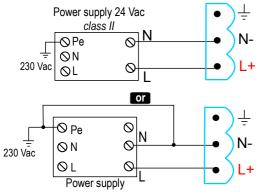
For transmitters with 115 or 230 Vac power supply:
